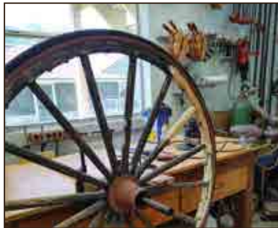
Wooden spokes needed to be restored.
